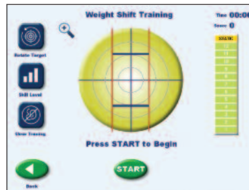
▲ WEIGHT SHIFT TRAINING - Patients are challenged to shift and control their center of gravity within two parallel lines, in the medial lateral, anterior posterior and transverse planes of movement. Changing the width of the lines controls the degree of difficulty. Score is kept to track progress.
