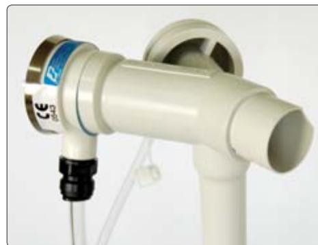
The new breathing valve can be easily disinfected and exchanged between tests.
